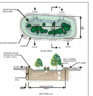
The diagram to the left shows a typical design of a bioretention system for use adjacent to a parking lot. In this application, precast car stops with gaps between them are used. An alternative is to use curbing with cuts to allow for water flow into the bioretention system (see photograph on Page 3).
