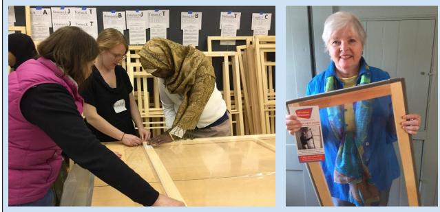
Each insert features a locally-sourced pine frame that is custom-built using the exact measurements of each window. This frame is wrapped tightly on both sides with polyolefin film, sealed, and finished with a foam gasket. Because our high-quality inserts are built by volunteers, they cost a fraction of commercial inserts. WindowDressers inserts create two insulating air spaces and perform better than commercially-available inserts that provide just one layer of insulation.
