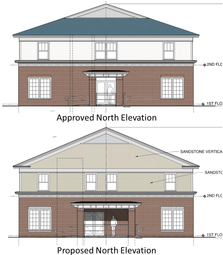
Figure 3. Image that shows the approved north elevation (top) and proposed north elevation (bottom) for the new mixed-use building.
