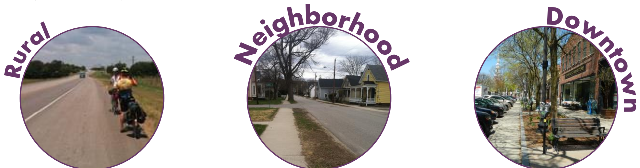
Examples of “Complete Streets.” Left: rural road with paved shoulder for bicyclists and walkers. Middle: neighborhood road with sidewalk, green buffer, and street trees. Right: downtown Main Street in Keene with a wide sidewalk, street trees/green buffer, street furniture, on-street parking, and outdoor café seating (not visible in picture).
